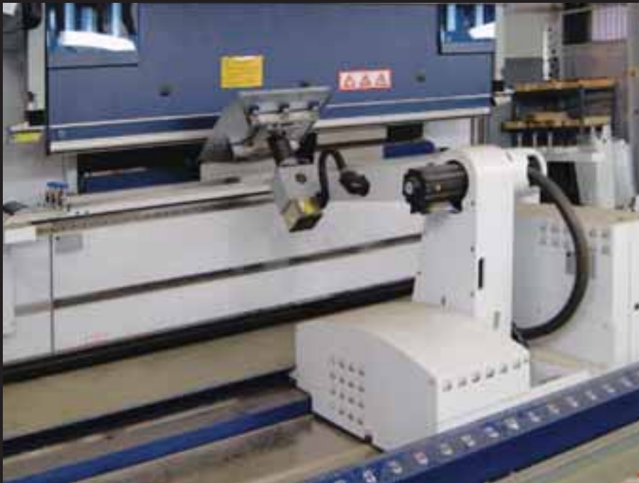
Robotized folding machine.
