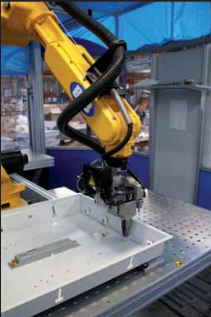
Robotized wiring cell.
