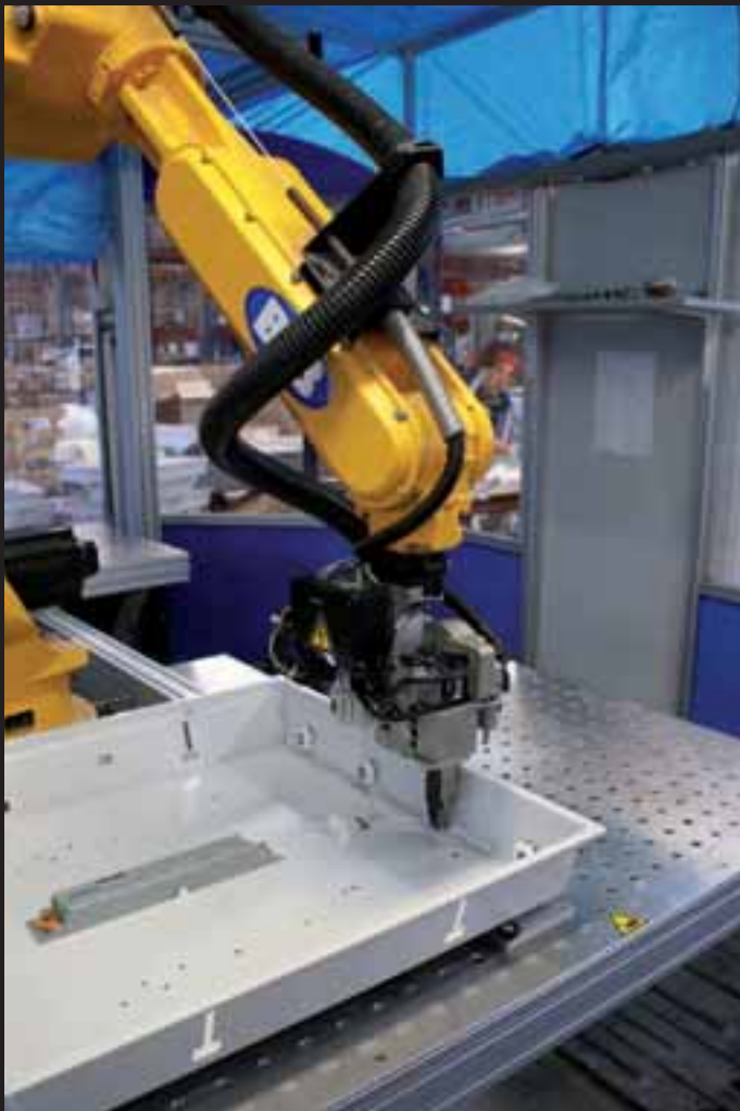
Robotized wiring cell.
