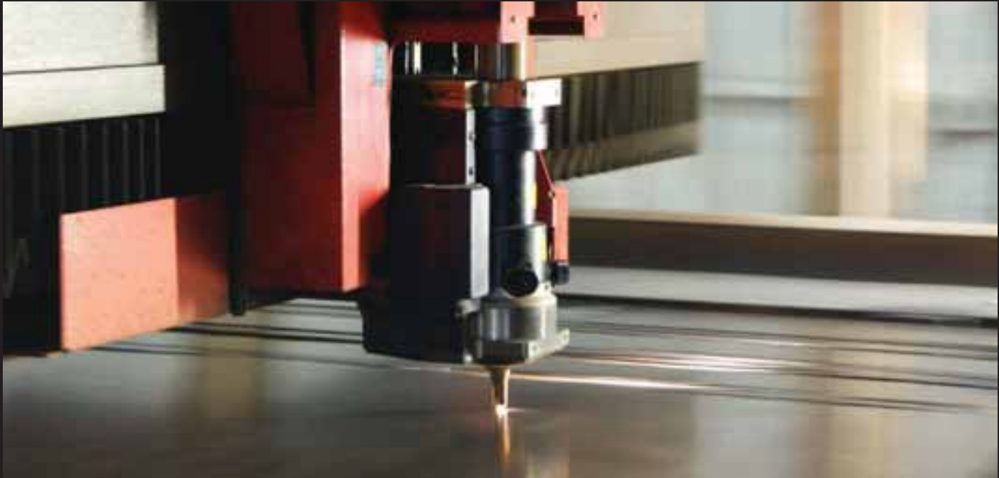
Laser cutting equipment for aluminum and other alloys for the manufacture of components.
