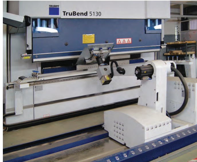
Robotized folding machine.
