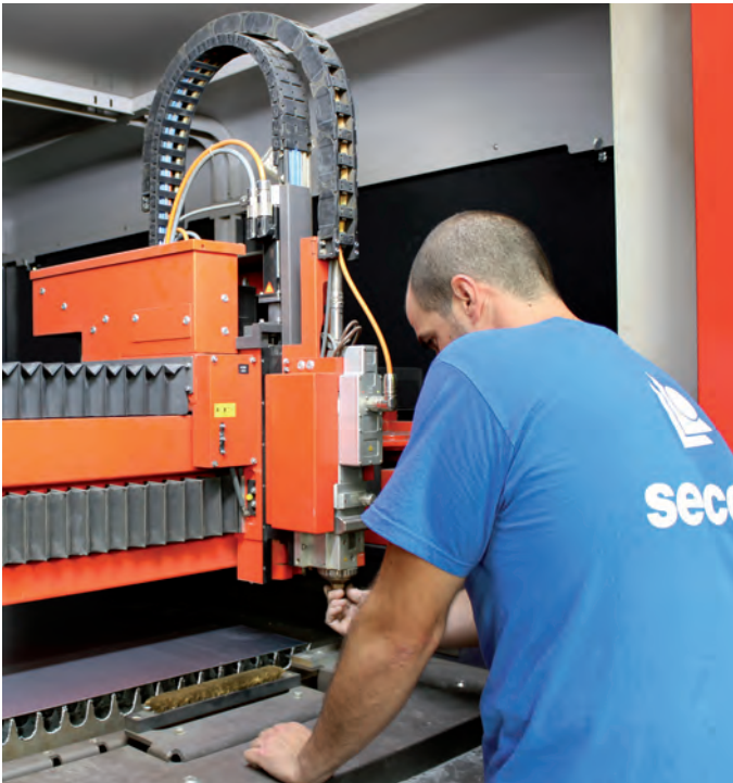
Laser cutting equipment for aluminum and other alloys for the manufacture of components.
