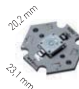
Osram LED DRAGON-X 1,2w a 350mA / Osram LED DRAGON-X 1,2w a 350mA
